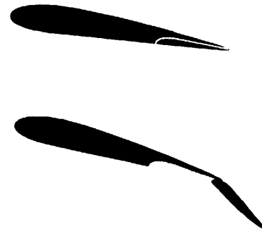
Fig 1-12 Fowler flap increases camber and wing area
